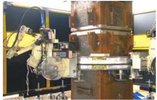
Manipulator-type onsite welding robot
