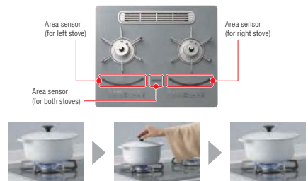
If a sleeve, etc. approaches the burner during cooking, the area sensor is activated to immediately reduce the flame to its lowest setting. When the sleeve, etc. is removed from the sensor, the flame returns to its previous strength. (Size of largest flame can be set manually)
