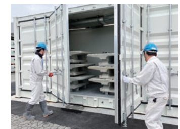
A CO 2 -SUICOM carbonation curing chamber
