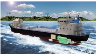
The Shimokita Maru equipped with a Kawasaki gas engine hybrid propulsion system
